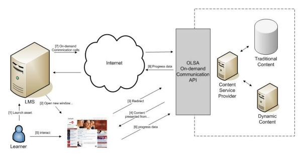
**Figure 1: System Architecture**
