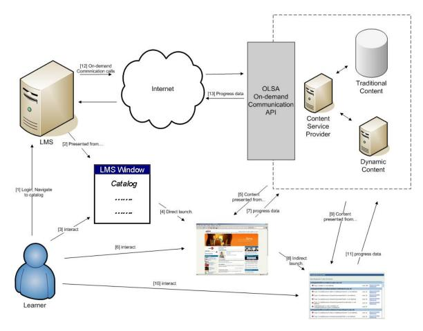
Figure 3: Data flow for Advanced Content
